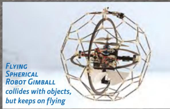
FLYING SPHERICAL ROBOT GIMBALL collides with objects, but keeps on flying
